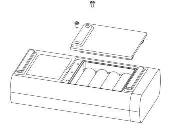
Figure 2 Installing Battery
